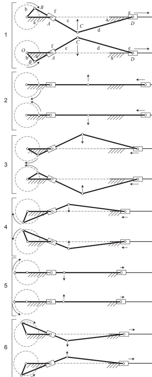
Figure 6: Sequence of motion of an antiphase tandem pair. (1→2→3→4→5→6→1→...)
