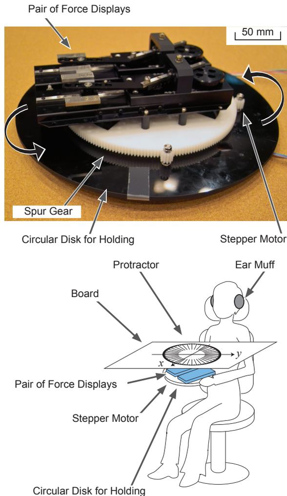
Figure 9: Photograph of the experimental apparatus (top) and a sketch of the view (bottom).
