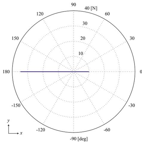
Figure 7: Change in the resultant force vector with the antiphase tandem pair of the force displays. The direction of the resultant force vector is limited to the x-axis. The mass of the slider is 40 g (20g each).
