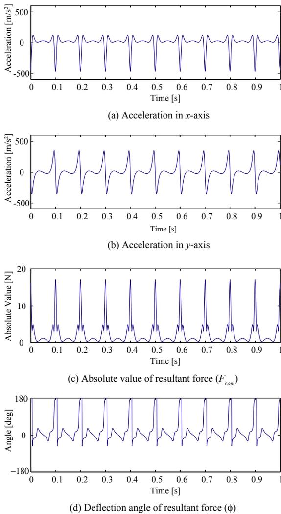
Figure 4: Characteristics of the force display when nongrounded. Frequency of the asymmetric acceleration is 10 Hz and the mass of the slider is 20 g.
