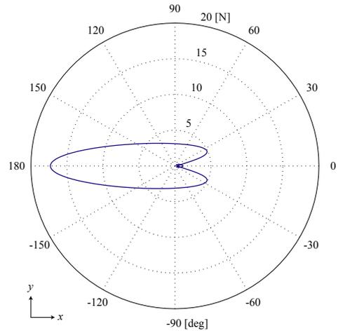
Figure 5: Change of the resultant force vector. The force direction covers not merely the  $x$ -axis but also the  $y$ -axis. The mass of the slider is 20 g.
