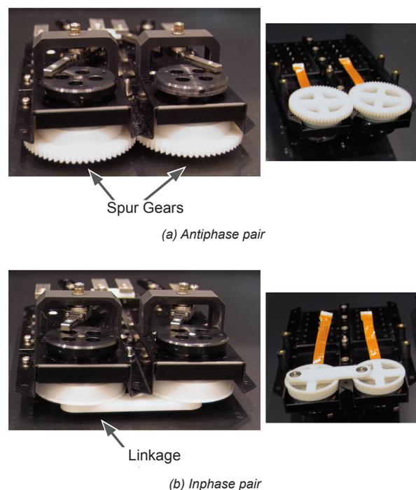
Figure 8: Photographs of the pairs of the force displays
