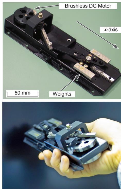
Figure 1: Photographs showing the force display utilizing the nonlinearity of human perception (top) and how it is held (bottom).
